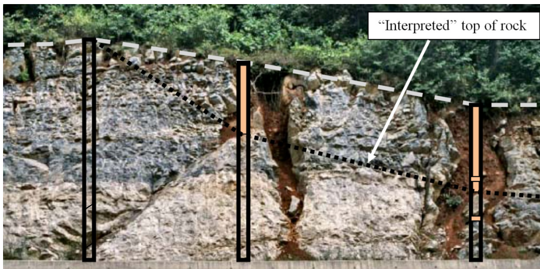
Figure 8. The perils of “connecting the dots” between drill holes in karst terrain. This photograph, taken from Waltham and Fooks 7 , has regularly spaced boreholes. The vertical development of karst shown in this rock cut means that simply drawing a line between adjacent boreholes can produce a substantially incorrect interpretation.
