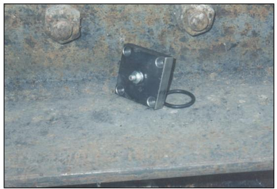
Photograph No. 5.—Front side of a grease block fitting.
