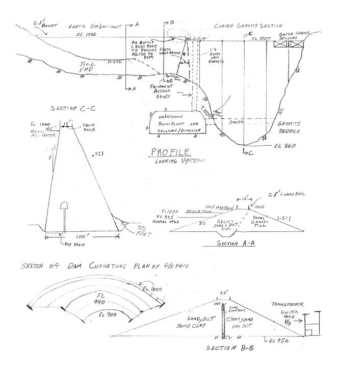
Figure A-3-1 Evans Creek Dam and Power Plant: Profile and Cross Sections
