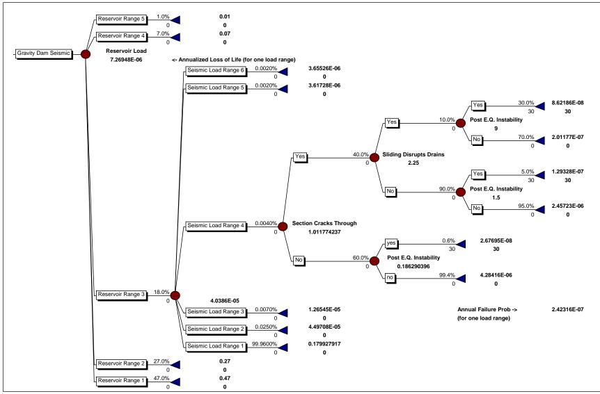
Figure E-3-3.—Concrete gravity dam instability, seismic loading.
