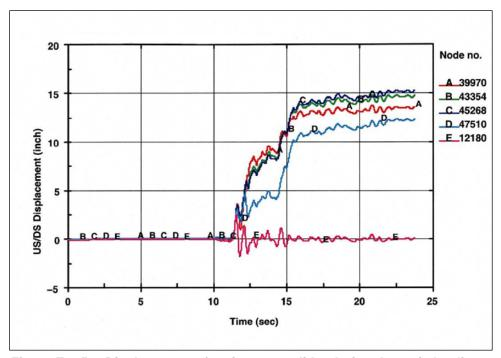
Figure E-3-5.—Displacement of various monoliths during dynamic loading (friction only, curve e is at base of sliding contact surface).
