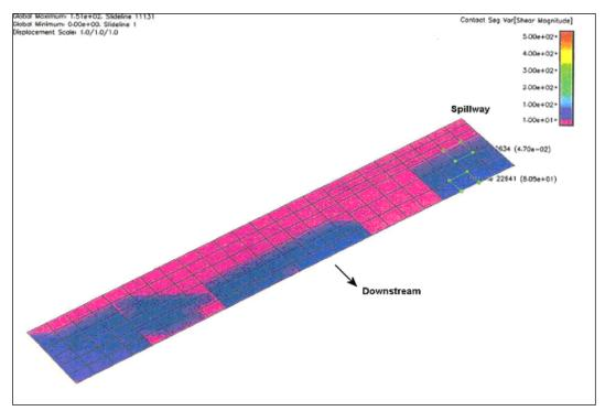
Figure E-3-4.—Separation of contact surface in dynamic finite element analysis (lighter color indicates separation).
