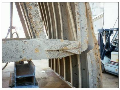
Figure G-2-15.—Failed culvert valve, Cannelton Locks and Dam.
