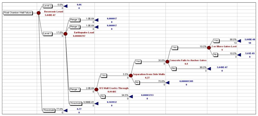
Figure G-2-12.—Example event tree for seismic failure of drum gate wall
