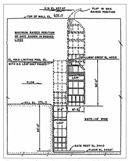
Figure G-2-6.—Submergible vertical lift gate (USACE 2006).
