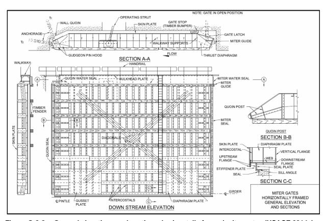
Figure G-2-8.—General elevations and sections, horizontally framed miter gates (USACE 2014a).
