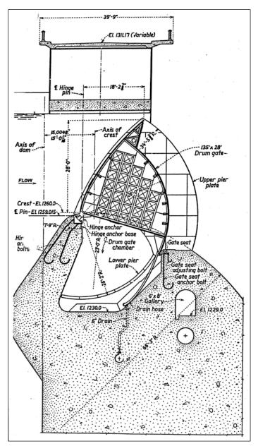
Figure G-2-1.—Cross section through drum gate.
