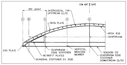
Figure G-2-16.—Vertical lift gate section at the arch frame, John Day Lock and Dam (USACE 1995).
