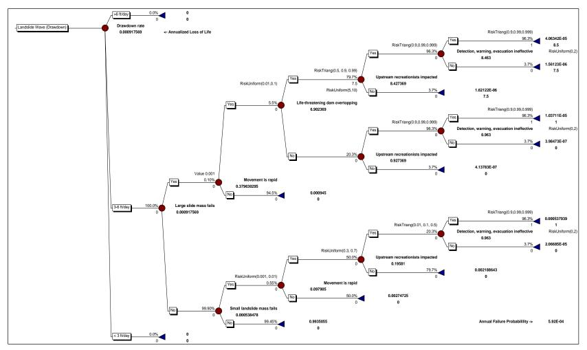
Figure H-2-1.—Example landslide event tree.
