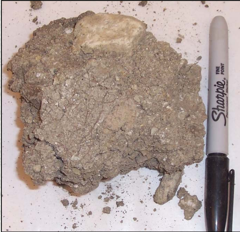
Embankment Soils – usually fine grained (clay silt)
