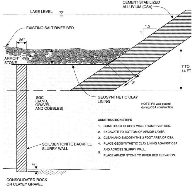
Figure 2. Cut-off Wall Section
