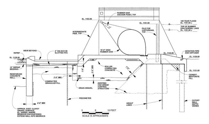
Figure 3. Downstream Dam Cross Section
