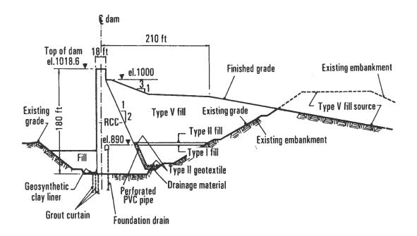
Typical Section of RCC Replacement Dam
