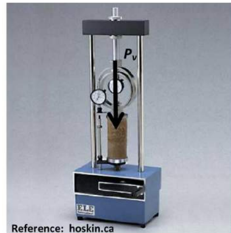
Figure 4: Unconfined compression test apparatus.
