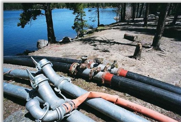
FIGURE 14 - FOUR SIPHONS IN PARALLEL OPERATION. THE PRIMING FITTINGS ARE SHOWN.
